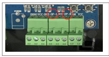
220V power to air switch , either port is ok
